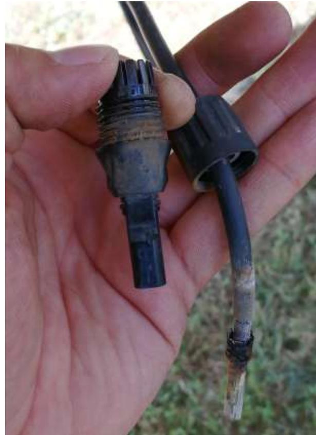
DC connectors melt due to the water goes inside as the cap has not been tightened, it damaged inverter in months after commissioning.
